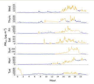
Fig. 8  $\sigma_{\Delta PM}$  filter applied to unit ccc9 for the first week in December 2021. Blue data points correspond to periods of low  $\sigma_{\Delta PM}$ , yellow data points correspond to periods of high  $\sigma_{\Lambda PM}$
