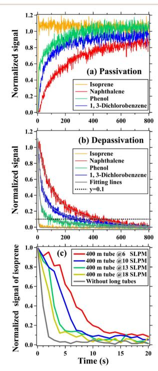
Fig. 1 (a) Passivation and (b) depassivation curves of four selected ion signals measured by PTR-ToF-MS for the 400 m long tubing at a flow rate of 13 SLPM. Ion signals were normalized to those measured at the start time of the step-function change; Grey solid lines in panel (b) are double exponential fittings. (c) Depassivation curves of isoprene for the 400 m long tubing at different flow rates.
