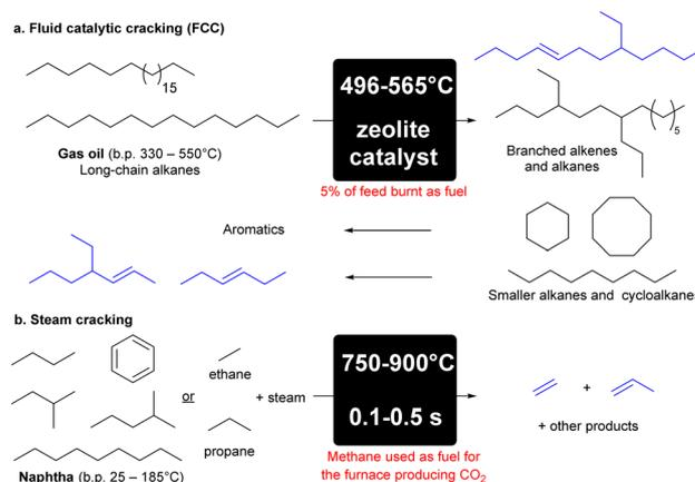
**Scheme 1** Cracking of hydrocarbons to produce alkenes via FCC (a) or steam cracking (b).<sup>8,9</sup>
