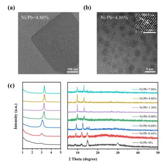
Fig. 2 HRTEM images of (a) the deep blue nanosheet and (b)  $FAPbBr_3$  QDs (Ni/Pb = 4.86%). Inset: Lattice distances of QDs. (c) XRD patterns of  $FAPbBr_3$  QDs (Ni/Pb = 0, 0.44, 0.60, 0.80, 1.36, 4.86 and 7.96%).
