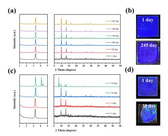
Fig. 4 FAPbBr<sub>3</sub> QDs with Ni/Pb = 4.86% thin films: (a) XRD patterns evolution, (b) images under 365 nm UV light. FAPbBr<sub>3</sub> QDs with Ni/Pb = 7.96% thin films: (c) XRD patterns evolution, (d) images under 365 nm UV light.
