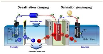
**Fig. 7** Seawater battery desalination (SWB-D). Reproduced with permission. <sup>176</sup> Copyright 2020, published by Elsevier.
