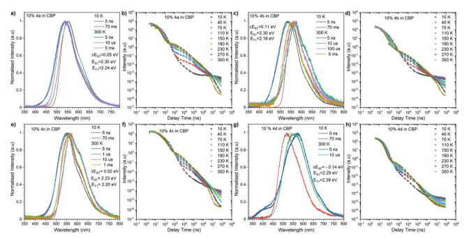
Fig. 3 Time-Resolved Spectra of compounds **4a-d** in CBP matrix (a, c, e and g), the energies correspond to the maximum emission peaks. Intensity vs delay time measurement decays (b, d, f and h).
