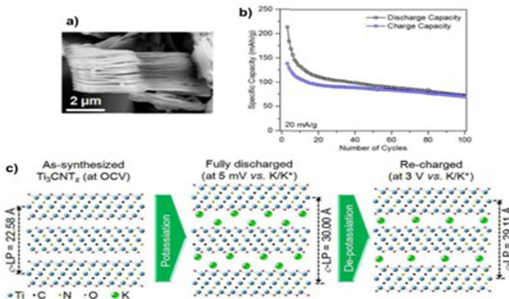
Fig. 7 (a) SEM Micrograph of  $\text{Ti}_3\text{CNT}_2$ . (b) Specific capacity vs. number of cycles at  $20 \text{ mA g}^{-1}$ . (c) Schematic representation of  $\text{Ti}_3\text{CNO}_2$  before and after electrochemical potassiation and de-potassiation. The image was adapted/reproduced from ref. 241 with permission from Chemical Communications 2017.
