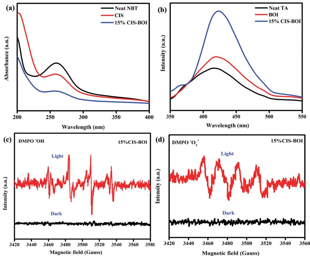
Fig. 13 (a) UV-vis spectra of pristine NBT, CIS, and CIS-BOI, and (b) PL spectra of pristine TA, BOI, and CIS-BOI. EPR spectra of 15% CIS-BOI under dark and light conditions: (c) DMPO- $\cdot\text{O}_2^-$  in methanol solution and (d) DMPO- $\cdot\text{OH}$  in water.
