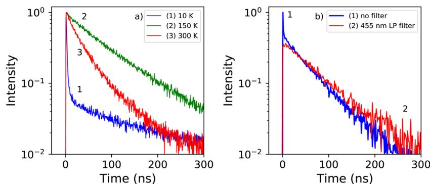
Fig. 5 (a) Temperature dependent X-ray excited decay spectra of  $\text{PEA}_2\text{PbBr}_4$  recorded at 10 K, 75 K, and 300 K. (b) X-ray excited decay spectra of  $\text{PEA}_2\text{PbBr}_4$  recorded at 10 K with and without 455 nm long pas filter.
