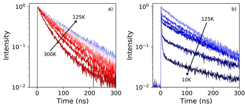
Fig. 6 (a) Temperature dependent X-ray excited decay spectra of  $\text{PEA}_2\text{PbBr}_4$  recorded from 125 K to 300 K, with a 25 K interval. The temperature decreases in the direction of the arrow. (b) Temperature dependent X-ray excited decay spectra of  $\text{PEA}_2\text{PbBr}_4$  recorded from 125 K to 25 K, with a 25 K interval, and at 10 K. The temperature decreases in the direction of the arrow.
