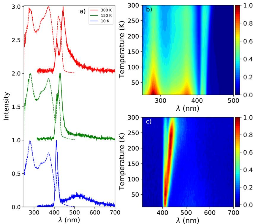
**Fig. 1** (a) Temperature dependent photoluminescence emission ( $\lambda_{\text{ex}} = 260$  nm) and excitation ( $\lambda_{\text{em}} = 530$  nm) spectra of  $\text{PEA}_2\text{PbBr}_4$ , from top to bottom: 300 K, 150 K, and 10 K. (b) Temperature dependent photoluminescence excitation spectra ( $\lambda_{\text{em}} = 530$  nm), from 300 K down to 10 K. (c) Temperature dependent photoluminescence emission spectra ( $\lambda_{\text{ex}} = 260$  nm), from 300 K down to 10 K.
