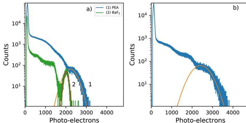
Fig. 8 Pulse height spectra recorded using a  $^{137}\text{Cs}$   $\gamma$ -source and a PMT as detector (a) Small, similar sized,  $\text{PEA}_2\text{PbBr}_4$  and  $\text{BaF}_2$ . (2 mm  $\times$  1 mm  $\times$  0.3 mm) (b) Large  $\text{PEA}_2\text{PbBr}_4$  crystal (8 mm  $\times$  5 mm  $\times$  1 mm).
