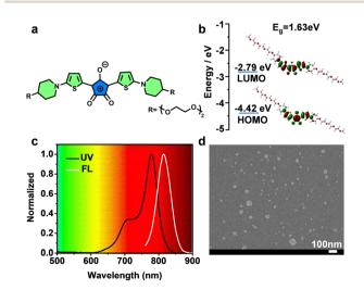
Fig. 1 Chemical structure (a) and molecular frontier orbitals of the ground state (b) of TCR. (c) Normalized UV-vis absorption and fluorescence spectra of TCR. (d) SEM image of TCR nanoparticles, scale bar: 100 nm.
