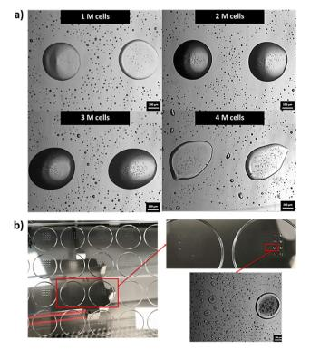
Fig. 4 (a) Influence of the cell concentration on the printability of 4% w/v H2SP-GelMA bio-inks; scale bar = 200  $\mu m$ . (b) Representative images of deposited droplets on tissue culture well plates; the increased probability of nozzle clogging occurs at higher cell concentrations (missing droplet on the left hand side as shown in the enlarged image).
