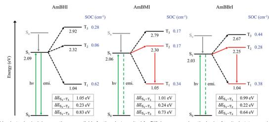
Fig. 3 Plausible photophysical decay pathways available for the photoexcited AmBXI dyes assessed on the basis of excited-state energies and spin-orbit coupling (SOC) values. The SOC values between the singlet  $S_1$  and the triplet  $T_m$  (m = 1-3) states are presented in blue. In the tables are listed the values of the energy gaps between the  $S_1$  and  $T_m$  (m = 1-3) states for each dye.
