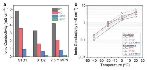
Fig. 2 (a) Total conductivity of the following electrolytes (STD1, STD2, and 2.5 m MPN) at room temperature,  $0^{\circ}$ C,  $-20^{\circ}$ C, and  $-40^{\circ}$ C. (b) Total conductivity estimated using molecular dynamics simulations ( $\bigcirc$ ) and measured experimentally ( $\triangle$ ). The relative magnitudes among the three systems are consistent between MD and experiment, as are temperature trends.
