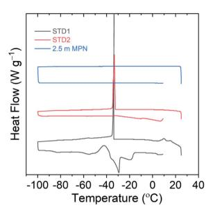
Fig. 3 Differential scanning calorimetry curves to identify possible freezing points using a scan range of 25  $^{\circ}$ C to -100  $^{\circ}$ C.
