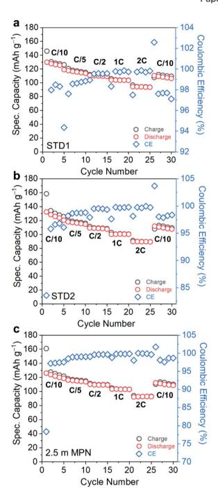
Fig. 4 Rate capability performance of  $gr\parallel LCO$  cells when subjected to C-rates ranging from C/10 to 2C and utilizing (a) STD1, (b) STD2, and (c) 2.5 m MPN electrolytes.
