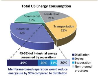
Fig. 5 Schematic of total US energy consumption and how membrane technology would reduce energy usage significantly (adapted by permission from Springer Nature: Nature, ref. 50, copyright 2016).
