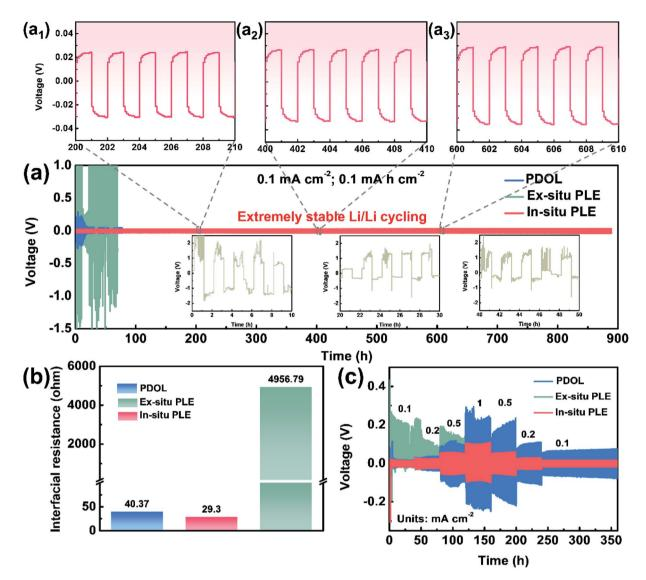
Fig. 3 Electrochemical characterization of different composite polymer electrolytes: (a) long-term cycling stabilities of symmetric cell; (a<sub>1</sub>-a<sub>3</sub>) enlarged voltage-time curves with periods of 200-210, 400-410 and 600-610 h. (b) Interfacial resistance ( $R_{ct}$ ) analyses before cycling. (c) Rate capabilities of Li|Li symmetrical cells
