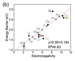
Fig. 8 Prediction of dehydrogenation energy barriers at MgH<sub>2</sub>/SACs-TM based on the linear correlation of dehydrogenation barrier vs. electronegativity. The empty and solid dots represent the predicted and DFT-calculated values, respectively. In (a), the elements consist of Sc and 5d TMs: TM = Sc, Y, Zr, Nb, Mo, Tc, Ru, Rh, Pd, and Ag. In (b), the elements consist of 4d TMs: TM = Hf, Ta, W, Re, Os, Ir, Pt, and Au.
