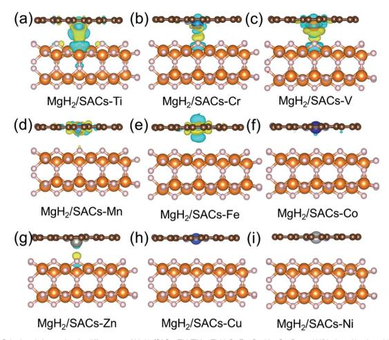
Fig. 5 (a-i) Calculated charge density differences of MgH $_2$ /SACs-TM (TM = Ti, V, Cr, Zn, Cu, Mn, Co, Fe, and Ni) induced by the addition of SACs. The yellow and blue isosurfaces indicate electron accumulation and loss, respectively. All the results are plotted with an isovalue of 0.001 e  ${\rm \mathring{A}}^{-3}$ . White, orange, brown, and gray spheres represent H, Mg, C, and N, respectively.
