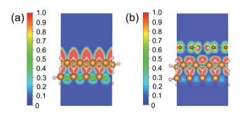
Fig. 4 ELFs of (a) MgH<sub>2</sub> and (b) MgH<sub>2</sub>/SACs-Ti. The section is the 010 plane of the H atom nearest to the metal atom. In the color bars, 1 represents a fully localized state, 0.5 represents a uniform electronic gas state, and 0 represents a fully nonlocalized state. The ELF results of other MgH<sub>2</sub>/SAC systems are shown in Fig. S4.†
