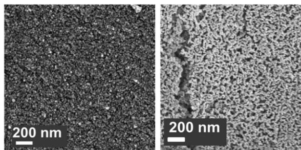
Fig. 3 Scanning electron micrograph of CaO stabilised with both MgO and Al<sub>2</sub>O<sub>3</sub> (left) as-synthesised and (right) after 23 cycles of carbonation/calcination.<sup>56</sup>
