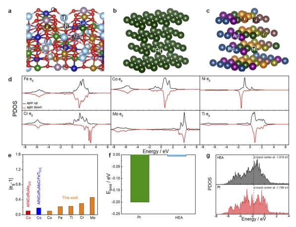
Fig. 4 (a) Computational models of (FeCoNiMoCrTi) $_3$ O $_4$  with a spinel structure, (b) pure Pt (111), and (c) HEA. (d) PDOSs onto the e $_g$  orbitals of the HEO sample. (e)  $|e_g-1|$  for metal elements in HEO and literature data. (f) Difference between  $\Delta E_O$  and the optimal value. The optimal value of  $\Delta E_O$  is 0.2 eV lower than  $\Delta E_O$  on Pt (111). (g) PDOS onto the Pt d orbitals of HEA and Pt (111). The black dashed lines indicate the d-band centers.
