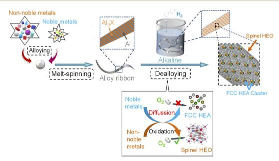
Scheme 1 Schematic illustration of the whole process for the preparation of the HEA nanoclusters supported on HEO.
