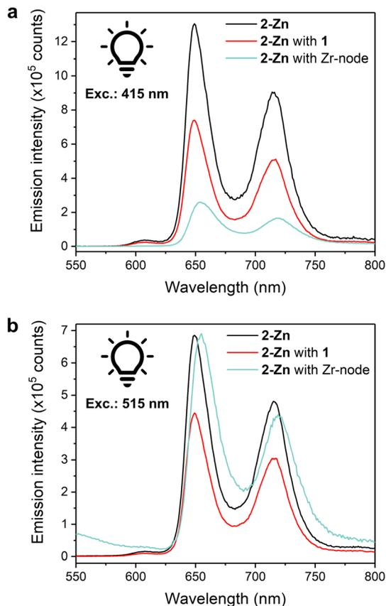
Fig. 5 Liquid-phase fluorescence spectra of MeCN/DMF (40/1 v/v) solutions containing **2-Zn** (0.05 mM), **2-Zn** (0.05 mM) and **1** (0.05 mM), and **2-Zn** (0.05 mM) with the isolated  $Zr_6$ -oxo-node (0.2 mM). (a) Excitation at 415 nm. (b) Excitation at 515 nm.
