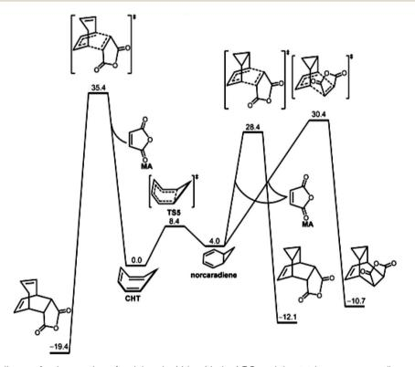
Fig. 10 The free energy diagram for the reaction of maleic anhydride with the 1,3,5-cycloheptatriene
