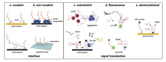
Fig. 3 Functional DNA-based detection strategies for small molecule environmental contaminants. (a) Covalent interfaces for aptasensors. (b) Non-covalent interfaces for aptasensors. (c) Colorimetric readouts for aptasensors. (d) Fluorescent readouts for aptasensors. (e) Electrochemical readouts for aptasensors.
