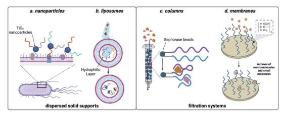
Fig. 5 Aptamer-based methods for sequestration of environmental contaminants. (a) Nanoparticle-based aptamer support. (b) Liposome-based aptamer support. (c) Aptamer column filtration. Reproduced from ref. 147, https://doi.org/10.1155/2017/3712070, under the terms of CC BY 4.0 license. (d) Aptamer membrane filtration.
