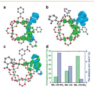
Fig. 4 Electron-hole distribution diagrams of (a) MIL-125, (b) MIL-125-NH<sub>2</sub> and (c) MIL-125-NO<sub>2</sub> in their excited states (red: O; sky blue: Ti; blue: N; gray: C; olive color: electrons; cyan color: holes). (d) Overlapping percentage and distance between electrons and holes in MIL-125 and MIL-125-X ( $X = NH_2$ ,  $NO_2$ ).
