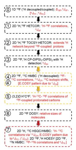
**Fig. 5** Flow chart for acquiring and working with spectra of mixtures of fluorinated compounds. The information obtained is given in red. Golden and red boxes denote experiments involving <sup>13</sup>C, and the experiments for extending the structure beyond the F-containing moieties, respectively.
