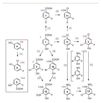
Fig. 6 Reaction pathways [1],  $^{94}$  [2],  $^{96}$  [3],  $^{50}$  and [4],  $^{95}$  identified in chloramination of **1**. Compounds enclosed in a rectangle fall outside of this classification. Fractions given represent concentrations relative to the starting material, **1**, as estimated from the intensity of signals in the 1D  $^{19}$ F NMR spectrum. \*unconfirmed intermediates, R = H or Cl.
