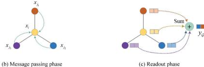
Fig. 3 Molecule representation and graph embedding. (a) Representing a molecule as a graph. (b) Graph message passing phase corresponding eqn (1). (c) Graph readout phase corresponding eqn (2).
