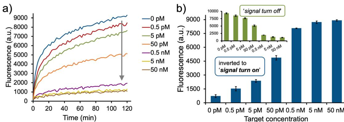
Fig. 1 Sensitivity of CRISPR-fHCR against different concentrations of dsDNA<sub>HBV</sub> depicted by (a) kinetic study 'signal turn off' and (b) end point fluorescence 'signal turn on'.
