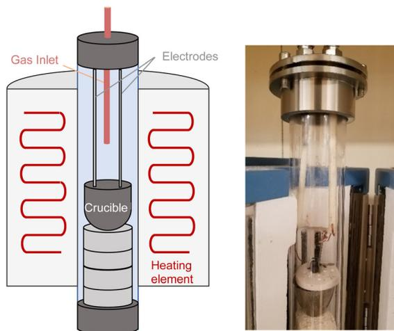
**Fig. 1** Schematic and photograph of the reactor for molten salt CO<sub>2</sub> electrolysis.
