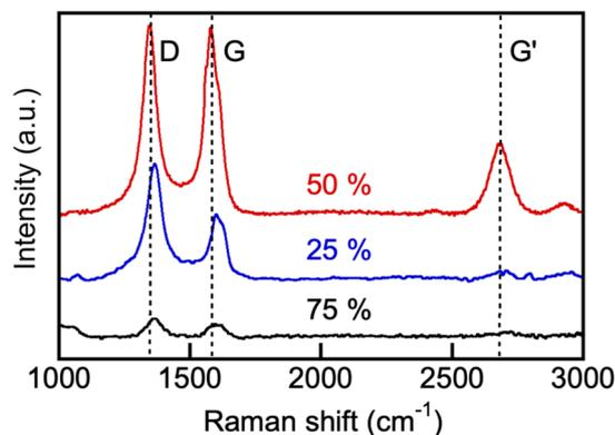
**Fig. 15** Raman spectra of the products of CO<sub>2</sub> electrolysis conducted in borate (Li<sub>1.5</sub>Na<sub>1.5</sub>BO<sub>3</sub>) and eutectic carbonate (Li<sub>1.24</sub>K<sub>0.76</sub>CO<sub>3</sub>) blends at 550 °C. Numbers indicate the initial borate concentration in the blend (mol%). For other detail, see Experimental.
