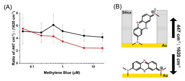
Fig. 6 (A) The ratio of the peaks at 447 cm<sup>-1</sup>:1620 cm<sup>-1</sup> for full silica (black) and end coated (red) AuNRs following exposure to varying amount of methylene blue. (B) A representation of the molecular orientation when the analyte is (top) in a pore and (bottom) not in a pore. The yellow represents the gold surface and the gray background represent the silica/pore channels.
