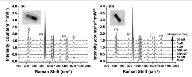
Fig. 3 Raman spectra taken for increasing methylene blue concentrations for the (A) full silica and (B) end silica coated gold nanorods. The spectra are offset for clarity. The large peak at 883 cm<sup>-1</sup> is the ethanol solvent peak. The methylene blue concentration range was from 0-20 μM. The numbers in the spectra correspond to the peak # in Table 1.
