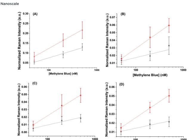
Fig. 5 The signal profile from 50-500 nM for the peaks at (A)  $447 \text{ cm}^{-1}$  (B)  $770 \text{ cm}^{-1}$  (C)  $1390 \text{ cm}^{-1}$  and (D)  $1620 \text{ cm}^{-1}$  for the AuNR@Full (black) and the AuNR@Ends (red). These points are fitted to a logarithmic equation and the slope was extracted to determine which concentration causes the SERS intensity to be higher than the intensity with no methylene blue added plus 3 standard deviations.
