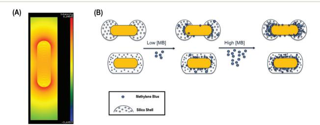
Fig. 1 (A) Logarithmically scaled electric field intensity map for the gold nanorods under excitation at the longitudinal plasmon band maximum. The map was made using nanoDDSCAT. The intensity was calculated assuming a solvent refractive index of 1.33, and the dipole spacing was set to 1.5 dipoles per nanometer. Red corresponds to the most intense electric field, blue the least. (B) Scheme of methylene blue (MB) adsorption to silica for the end-capped silica AuNRs vs. the fully coated AuNRs.
