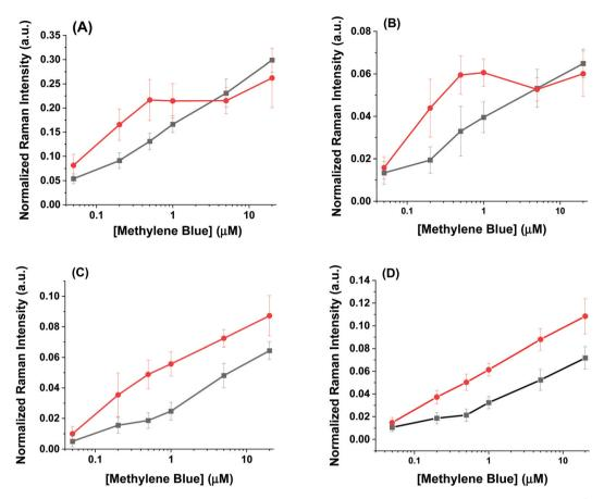
Fig. 4 Normalized intensity of different methylene blue Raman peaks relative to internal ethanol Raman peaks for (A) 447 cm<sup>-1</sup> (B) 770 cm<sup>-1</sup> (C) 1390 cm<sup>-1</sup> (D) 1620 cm<sup>-1</sup>. The AuNR@Full and the AuNR@Full an
