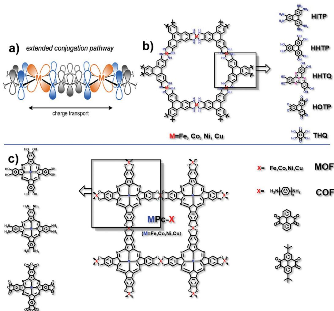
**Fig. 3** (a) Charge transport pathway of extended conjugation. This figure has been adapted from ref. 17 with permission from the American Chemical Society, copyright 2020; (b) structure of HITP analog based MOFs; and (c) structure of MPC-X, matching metals (for MOFs) and organic ligands (for COFs).
