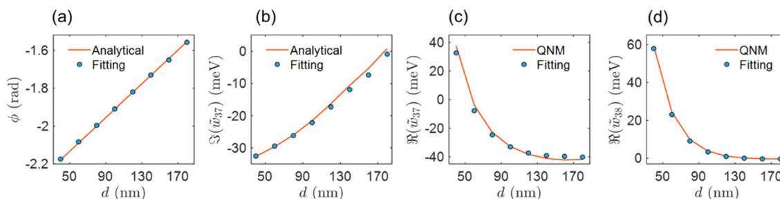
**Fig. 4** Comparison between fitting parameters and analytical results. Analytical  $\phi$  (a) and  $\Im(\tilde{\omega}_{37})$  (b) from eqn (S15.3) and (S19.9)<sup>†</sup> are found to be almost identical to their fitted counterparts. In addition, the near field coupling coefficients deduced from the QNM field overlapping integral coincide well with  $\Re(\tilde{\omega}_{37})$  (c) and  $\omega_{38}$  (d).
