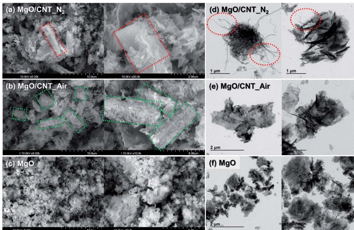
Fig. 2 SEM and TEM images of pristine MgO sorbents. SEM images of (a) MgO/CNT<sub>N<sub>2</sub></sub>, (b) MgO/CNT<sub>Air</sub>, and (c) MgO samples, and TEM images of (d) MgO/CNT<sub>N<sub>2</sub></sub>, (e) MgO/CNT<sub>Air</sub>, and (f) MgO. Dotted areas in red and in green indicate CNT with MgO flakes, and tubular-shaped MgO flakes without CNT, respectively.
