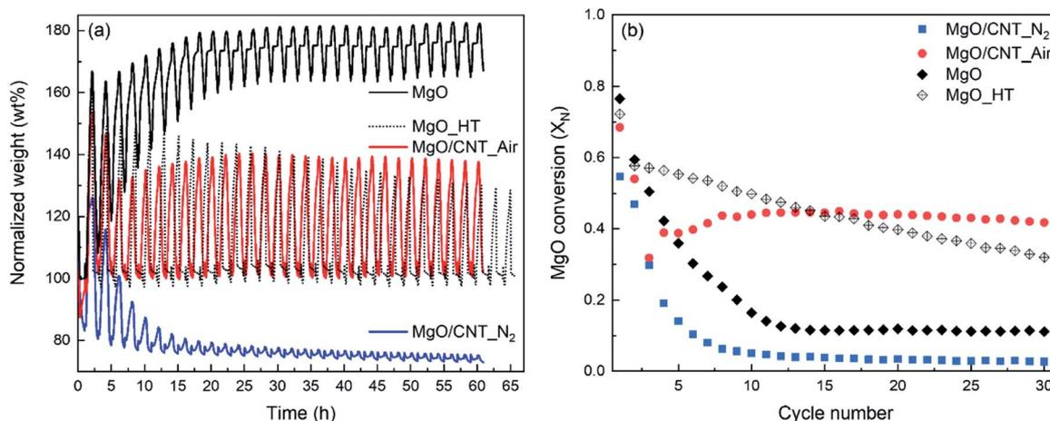
Fig. 3 CO<sub>2</sub> capture performance of MgO-based sorbents for 30 cycles of carbonation–dissociation measured by TG–DSC. (a) Normalized weight (wt%) profiles and (b) MgO conversion ( $X_M$ ). Weight profiles are normalized according to each weight of pristine MgO-based sorbents.
