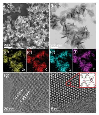
Fig. 1 (a) SEM, (b) TEM, (c)-(f) EDS mapping, (g) high-resolution TEM, and (h) STEM iDPC images (inset shows the corresponding structure) of UiO-66-F<sub>4</sub>.
