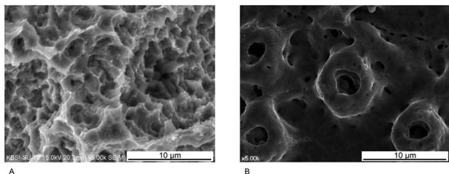
**Fig. 4** (A) Scanning electron microscopy (SEM) image of a hydrophilic SLA surface (SLActive, Institute Straumann AG, Basel, Switzerland). There are no distinct differences in specific SEM features between hydrophilic and standard SLA surfaces. (B) SEM images of an anodically oxidized Ti surface (TiUnite, Nobel Biocare, Zürich, Switzerland) displaying protruded open pore micro-structures.
