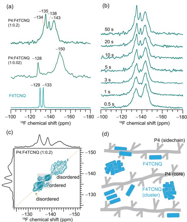
**Fig. 5** Solid-state (a) 1D  $^{19}\text{F}$  MAS NMR spectra of the neat F4TCNQ and P4:F4TCNQ blends with different F4TCNQ molar ratios, and (b)  $T_2$ -filtered  $^{19}\text{F}$  MAS NMR spectra of P4:F4TCNQ (1:0.2) as a function of spin-echo time, and (c) 2D  $^{19}\text{F}$ - $^{19}\text{F}$  spin-diffusion NMR spectrum of P4:F4TCNQ (1:0.2) acquired with  $500$  ms mixing time. (d) Schematic representation of different distributions of F4TCNQ molecules in the P4 polymer chains.
