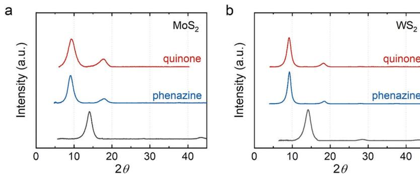
Fig. 4 XRD of electron-proton transfer mediator intercalated (a) MoS<sub>2</sub> and (b) WS<sub>2</sub>. Red: *p*-benzoquinone-intercalated; blue: phenazine-intercalated; dark gray: restacked.
