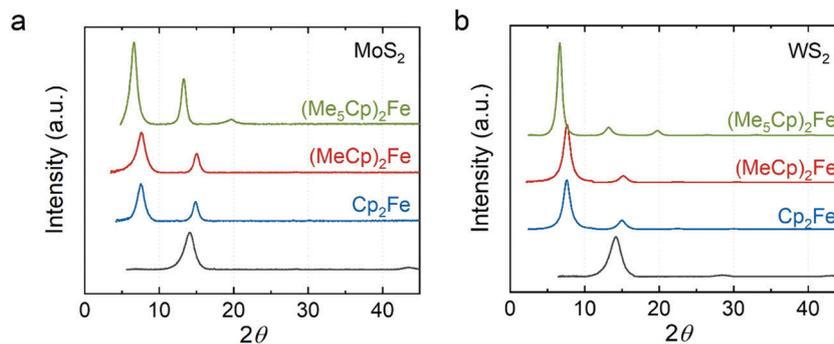
Fig. 2 XRD of metalocene intercalated (a) MoS<sub>2</sub> and (b) WS<sub>2</sub>. Green: decamethylferrocene-intercalated; red: 1,1'-dimethylferrocene-intercalated; blue: ferrocene-intercalated; dark gray: restacked.
