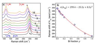
**Fig. 6** (a) Raman spectra of CANBIC perovskites with varied Bi fraction y=0 (1), 0.01 (2), 0.05 (3), 0.07 (4), 0.10 (5), 0.15 (6), 0.20 (7), 0.50 (8), 0.80 (9), and 1.00 (10). (b) Frequency of the  $A_{1g}$  mode as a function of Bi fraction y (scatter). Solid red line represents the best fit with a polynominal function " $\nu(A_{1g})$  versus y" presented in the figure.
