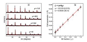
**Fig. 2** (a) X-Ray diffractograms of CANBIC perovskites with x = 0.4 and y = 0, 0.2, 0.5, and 1.0. Gray circles correspond to experimental data, red solid lines are the results of Rietveld refinement. (b) Cell parameter of CANBIC perovskites as a function of Bi fraction y. Gray squares are experimental data, red line represents a linear fit (fitting parameters a and b are presented in figure).
