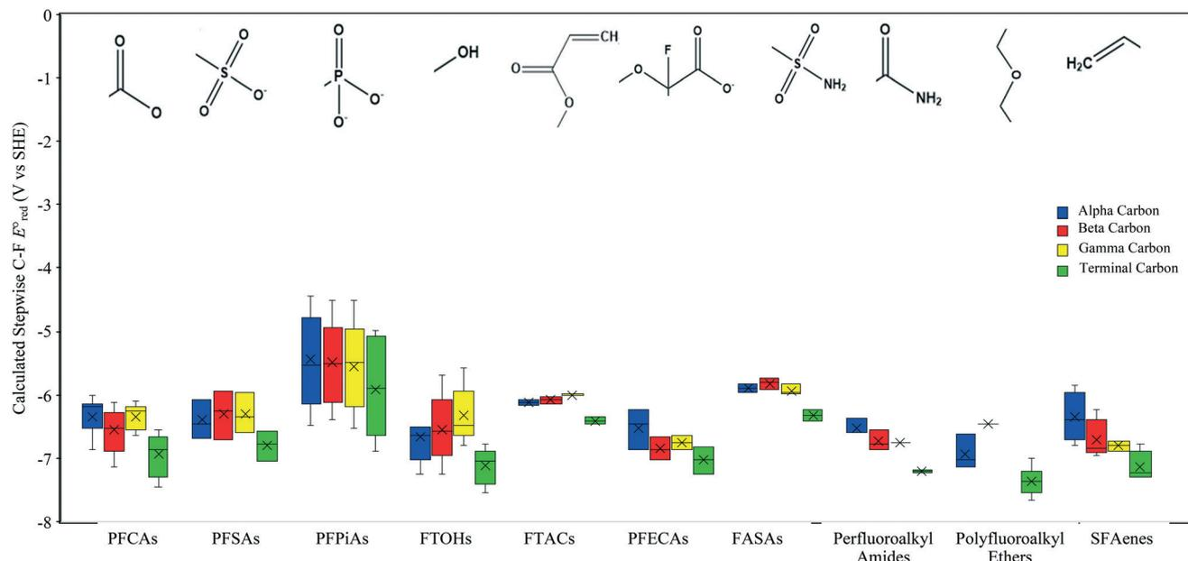
Fig. 4 Theoretically calculated  $E_{\text{red,eq}}^{\circ}$  values for the cleavage of a C-F bond at different positions of various PFASs. The  $E_{\text{red,eq}}^{\circ}$  values were calculated based on M06-2X/cc-pVDZ.
