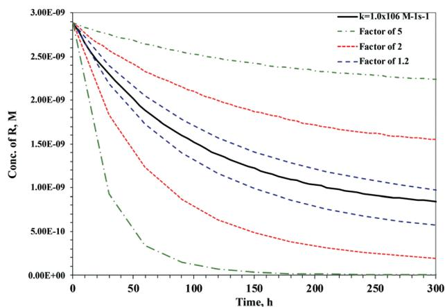
Fig. 5 Time-dependent concentration of a target compound with  $k_{\text{chem}} = 1.0 \times 10^6 \text{ M}^{-1} \text{ s}^{-1}$  and different predicted values by a difference of a factor of 1.2, 2, and 5 in UV/sulfite process.<sup>10</sup>
