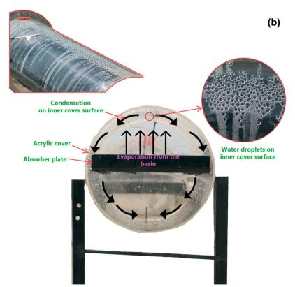
Fig. 2 (a) Photograph of the TSS experimental test set-up without CF, functionalized with CF, and functionalized with the CF modified with candle soot derived carbon nanoparticles, (b) photographic view of water droplets condensing on the cover of the TSS.
