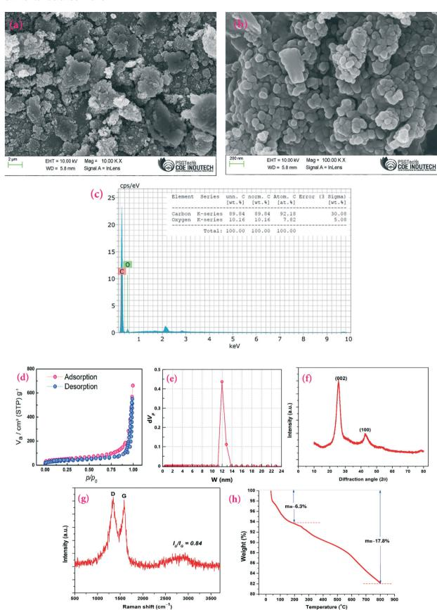
Fig. 3 Characterization of the produced CSCNP using SEM micrographs at magnifications of (a) 2 µm and (b) 200 nm; (c) EDX analysis showing the percentage of the elements present; (d) N2 adsorption/desorption isotherm; (e) NLDFT/GCMC pore size distribution analysis; (f) XRD diffractogram; (g) Raman spectrum; and (h) thermogravimetric analysis.
