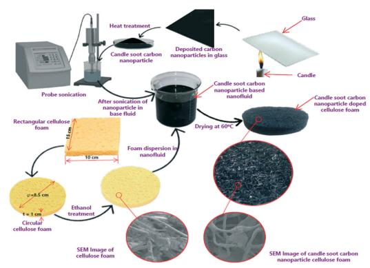
Fig. 1 Preparation route of candle soot carbon nanoparticles (CSCNPs) and their deposition onto cellulose foam (CF).
