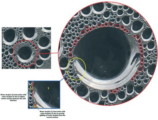
Fig. 10 Mechanism of larger droplet formation due to van der Waals interactions between the water molecules. A movie of this processes is included in the ESI.†
