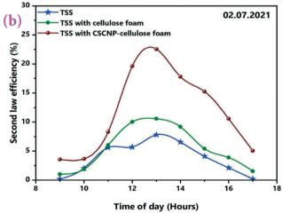
Fig. 13 Second law efficiency of different TSS on (a) 1st and (b) 2nd July, 2021.
