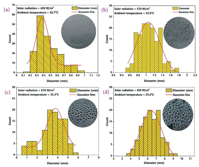
Fig. 9 Effect of varying solar radiation intensity on the condensed water-droplet formation inside the cover of the CSCNP-CF-TSS. (a) 430 W m<sup>-2</sup>, (b) 570 W m<sup>-2</sup>, (c) 810 W m<sup>-2</sup> and (d) 830 W m<sup>-2</sup>. The insets show the actual droplet sizes (photographs).
