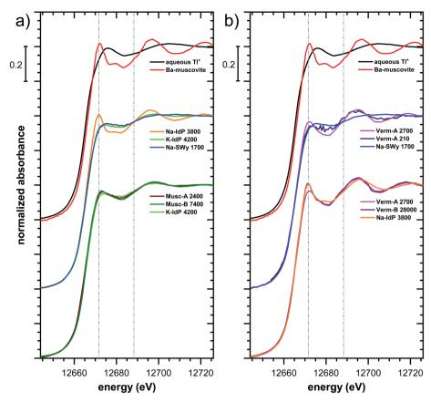
Fig. 5 Comparison of the Tl L<sub>III</sub>-edge XANES spectra of selected Tl-loaded phyllosilicate samples. Numbers in spectra labels indicate the Tl loading of the respective phyllosilicate in mg kg<sup>-1</sup>. Vertical lines serve to guide the eye. An enlarged version of figure focusing on post-edge oscillations is provided in Fig. S16.†
