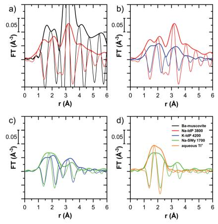
Fig. 6 Fourier-transformed  $k^2$ -weighted Tl L<sub>III</sub>-edge EXAFS spectra of Tl-containing Ba-muscovite, Tl-loaded Na-IdP and K-IdP, Na-SWy and of aqueous Tl<sup>+</sup>; sequentially pair-wise compared (a-d; thick lines indicate magnitude, thin lines imaginary part). Numbers in sample names indicate the Tl loading of the phyllosilicates in mg kg<sup>-1</sup>.
