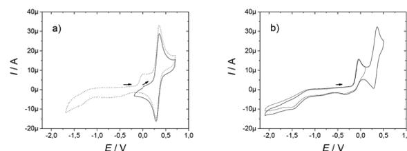
**Fig. 1** CV curves of 0.5 mM CH<sub>3</sub>CN solutions (+0.1 TBAP) of (a) **L**<sub>1</sub> and (b) **L**<sub>2</sub> at a carbon electrode.  $T$  = 298 K, scan rate = 0.1 V s<sup>-1</sup>. All values reported with respect to the regular Fc<sup>+/0</sup>/Fc redox couple that was used as an external reference.
