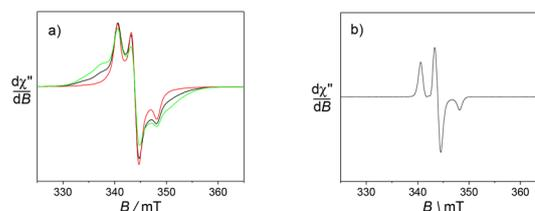
Fig. 5 X-band EPR spectra of 0.45 mM aqueous solutions (+10% glycerol) of (a)  $[\text{Yb}(\text{L}_1)]^{3+}$  and (b)  $[\text{Yb}(\text{L}_2)]^{3+}$ . Microwave freq. 9.63 GHz; power 0.8 mW; mod. amp. 0.4 mT, freq. 100 KHz; (a)  $T = 4$  (green), 10 (black), 20 (red) K; (b)  $T = 10$  K.
