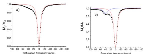
**Fig. 7** Z spectra of a 20 mM H<sub>2</sub>O : CD<sub>3</sub>CN (2 : 1) solution of [Eu(L<sub>2</sub>)]<sup>3+</sup> in a HEPES buffer (0.07 M, pH 7.4) under its hydroxylamine form generated by chemical reduction using 2 eq. of sodium ascorbate. (a)  $T = 298$  K, (b)  $T = 310$  K.  $B_0 = 11.7$  T,  $B_1 = 19$   $\mu$ T, irradiation time = 4 s.
