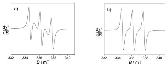
Fig. 4 X band EPR spectra of 0.5 mM  $\text{CH}_3\text{CN}$  solutions of the ligands (a)  $\text{L}_1$  and (b)  $\text{L}_2$ . Microwave freq. 9.42 GHz; power, 3.5 mW; modulation amp., 0.2 mT; freq. 100 KHz.  $T = 293$  K.
