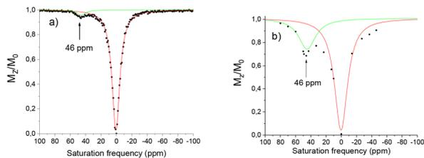
**Fig. 6** Z spectra of a 20 mM H<sub>2</sub>O : CD<sub>3</sub>CN (2 : 1) solution of [Eu(L<sub>1</sub>)]<sup>3+</sup> in a HEPES buffer (0.07 M, pH 7.4). (a) Nitroxide form, (b) hydroxylamine form generated by chemical reduction using 2 eq. of ascorbate.  $B_0 = 11.7$  T,  $B_1 = 25$   $\mu$ T, irradiation time = 4 s,  $T = 298$  K.
