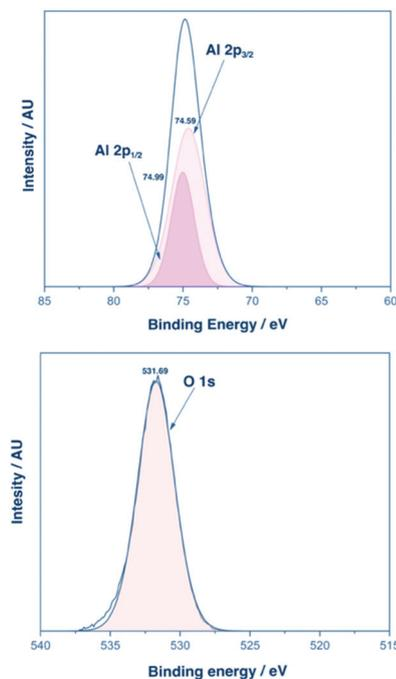
Fig. 5 XPS analysis of an  $\alpha$ -Al<sub>2</sub>O<sub>3</sub> film deposited from complex **3-Al**. Top: XPS of the Al 2p<sub>1/2</sub> and 2p<sub>3/2</sub> states. Bottom: XPS of the O 1s state.
