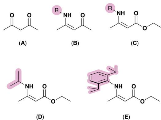
**Fig. 1** Top: previously reported ligand systems for oxide formation include  $\beta$ -diketones (A),  $\beta$ -diketoinimines (B) and aminoenoates (C). Bottom: the aminoenoate pro-ligands employed in this work with  $i$ -Pr (D) and  $-Dip$  (2,6-diisopropylphenyl) (E) at the N-position. R-groups that can be tuned to vary precursor geometry, highlighted in pink.
