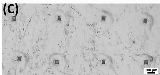
Fig. 5 Insertion test in the Parafilm® skin simulant model. (A) The side length of the pores created by MNs on the first two Parafilm® layers ( n = 10 , mean \pm s.d.). Representative microscopic images of Parafilm® into which FUR-MN2 was inserted: (B) first layer (140 μm), (C) second layer (280 μm). Scale bar 100 μm.
