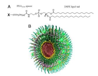
Fig. 3 Construction of modular multifunctional micelles. (A) Individual lipopeptide monomers are made up of a DSPE tail, a poly (ethylene glycol) (PEG2000) spacer, and a variable polar head group (X) of CREKA, FAM-CREKA, FAM, N-acetylcysteine, Cy7, or hirulog. The monomers were combined to form various mixed micelles. (B) The 3D structure of FAM-CREKA/Cy7/hirulog mixed micelle. Adapted with permission from ref. 84. Copyright (2009) PNAS.
