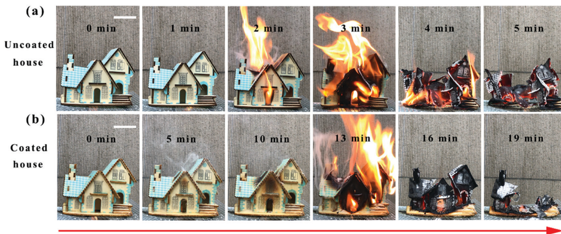
Fig. 4 Application of the biogel coating on wooden house models. Wooden house models without (a) and with (b) the biogel coating during combustion. Scale bar, 5 cm.
