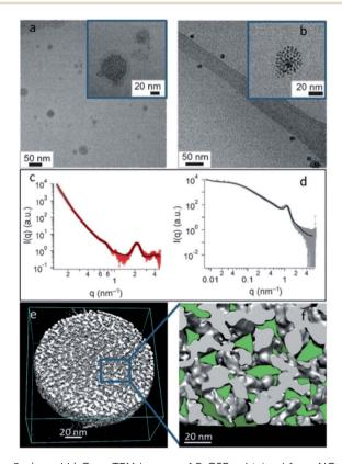
Fig. 5 (a and b) Cryo-TEM images of F-GSPs obtained from NCs (a) and NPs (b). (c and d) SAXS pattern and corresponding fit of F-GSPs obtained from NC (c) and NP (d) self-assembly. (e) ET3D reconstruction of an F-GSP obtained from NPs, and (f) an ET 3D enlargement with confined spaces forming fluorinated pockets marked in green. Reproduced with permission from ref. 75. Copyright 2017 Wiley and Sons.
