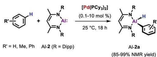
Scheme 3 (a) Reaction of [Pd(PCy<sub>3</sub>)<sub>2</sub>] with Al-2. (b) Catalytic aluminium of benzene.
