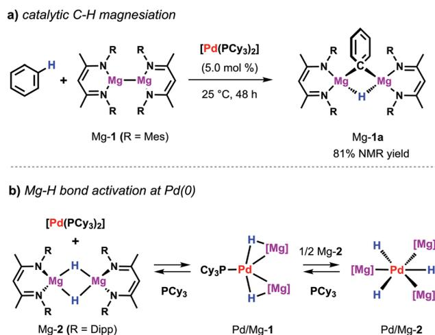
Scheme 9 (a) Pd-catalysed magnesiation of benzene. (b) Stoichiometric reactivity of [Pd(PCy<sub>3</sub>)<sub>2</sub>] with Mg-2.
