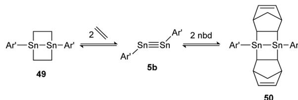
Scheme 25 Reversible cycloaddition of ethylene to distannyne **5b**. Ar' = C<sub>6</sub>H<sub>3</sub>-2,6-(C<sub>6</sub>H<sub>3</sub>-2,6-*i*-Pr<sub>2</sub>)<sub>2</sub>, nbd = norbornadiene.<sup>138</sup>
