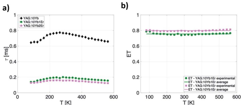
**Fig. 6** (a) Temperature dependence of the  ${}^2\text{F}_{5/2}$  lifetime for YAG:10Yb1Er, YAG:10Yb2Er and YAG:10Yb samples and (b) temperature-dependence of  $\text{Yb}^{3+} \rightarrow \text{Er}^{3+}$  energy transfer.
