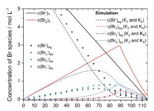
Fig. 10 Comparison of polybromide concentrations from measurements (dots) with simulated values based on polybromide equilibria from the literature (dashed line) next to global and equilibrium concentrations of bromine (red – line and dashed line) and HBr (black – line, dots and dashed line).
