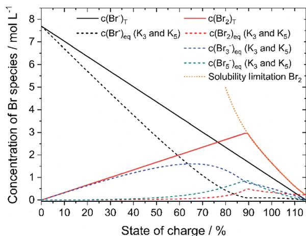
Fig. 7 Plot of the theoretical concentration of  $\text{HBr}_T$ ,  $\text{Br}_{2,T}$ ,  $\text{Br}_{3,\text{eq}}^-$ ,  $\text{Br}_{5,\text{eq}}^-$  with  $K_3 = 16 \text{ L mol}^{-1}$  and  $K_5 = 37 \text{ L}^2 \text{ mol}^{-2}$  including bromine solubility limit.
