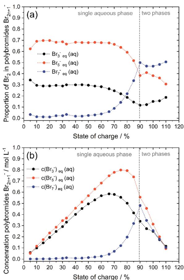
Fig. 9 (a) Distribution of bromine on different polybromides  $x(\text{Br}_3^-)$ ,  $x(\text{Br}_5^-)$  and  $x(\text{Br}_7^-)$  for the investigated electrolyte mixture as a function of SOC and (b) polybromide concentrations as a function of SOC for the investigated electrolytes.
