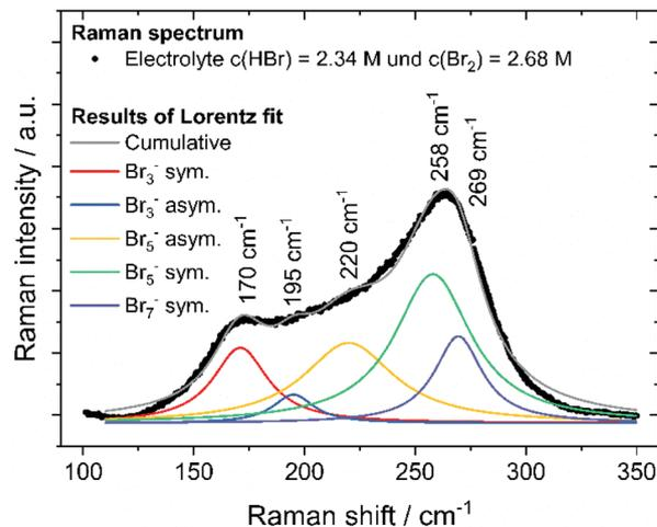
Fig. 8 Raman spectrum of the electrolyte mixture with  $c(\text{HBr}) = 2.34$  M and  $c(\text{Br}_2) = 2.68$  M (SOC = 80%) and water including Raman fitting for the symmetrical and antisymmetrical stretching oscillation of tribromide, pentabromide and heptabromide.
