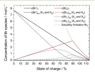
Fig. 7 Plot of the theoretical concentration of HBr $_T$ , Br $_{2,T}$ , Br $_{3,eq}^-$ , Br $_{5,eq}^-$  with  $K_3=16$  L mol $^{-1}$  and  $K_5=37$  L $^2$  mol $^{-2}$  including bromine solubility limit.
