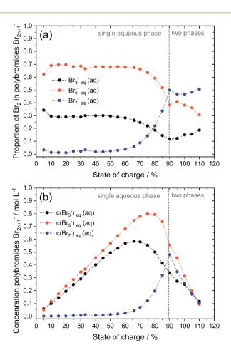
Fig. 9 (a) Distribution of bromine on different polybromides  $x(Br_3^-)$ ,  $x(Br_5^-)$  and  $x(Br_7^-)$  for the investigated electrolyte mixture as a function of SOC and (b) polybromide concentrations as a function of SOC for the investigated electrolytes.
