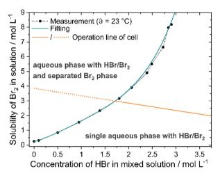
Fig. 5 Solubility of  $Br_2 \ c(Br_2)_{sat}$  in aqueous HBr solutions  $c(HBr)_{sat}$  as a function of the HBr concentration in the solution (black dots and green fitting line) and superposition with the operation line (orange line) of the  $H_2/Br_2$ -RFB electrolyte by stoichiometric concentration change.
