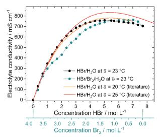
Fig. 6 (a) Electrolyte conductivities as a function of the concentration of HBr c(HBr) in a pure HBr solution and HBr/Br $_2$  solution for a bromine half cell. Measurements shown as points and literature values as lines [11,53] and (b) quantitative ratio between water H $_2$ O and HBr in the investigated electrolyte solutions as a function of the HBr concentration.
