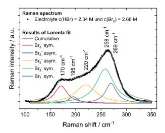
Fig. 8 Raman spectrum of the electrolyte mixture with c(HBr) = 2.34 M and  $c(Br_2) = 2.68 \text{ M}$  (SOC = 80%) and water including Raman fitting for the symmetrical and antisymmetrical stretching oscillation of tribromide, pentabromide and heptabromide.
