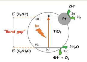
Fig. 1 Schematic diagram of the water-splitting reaction on Pt/TiO<sub>2</sub> as a heterogeneous photocatalyst.
