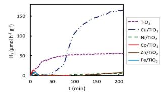
Fig. 3 Hydrogen production for 2 wt% impregnated M/TiO<sub>2</sub> photocatalysts (M = Fe, Co, Ni, Cu, Zn) under visible lamp irradiation.
