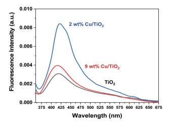
Fig. 11 Photoluminescence spectra of the obtained bare  $TiO_2$  and titania modified with Cu (2 and 9 wt%), when excited at 340 nm.
