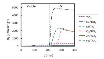
Fig. 2 Hydrogen production for impregnated M/TiO<sub>2</sub> photocatalysts (M = Fe, Co, Ni, Cu, Zn), 2 wt% M, under both visible and UV light
