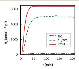
Fig. 6 Comparison of the catalytic activity of bare commercial  ${\rm TiO_2}$ , 2 wt%  ${\rm Cu/TiO_2}$  and 2 wt%  ${\rm Pt/TiO_2}$  in the hydrogen photoproduction under UV irradiation.
