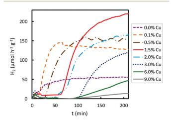
Fig. 5 Effect of Cu impregnated content of TiO<sub>2</sub> on photocatalytic hydrogen production under visible light irradiation.
