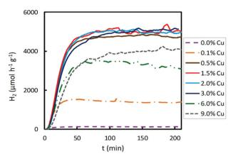
Fig. 4 Effect of Cu content on photocatalytic hydrogen production under UV light irradiation.
