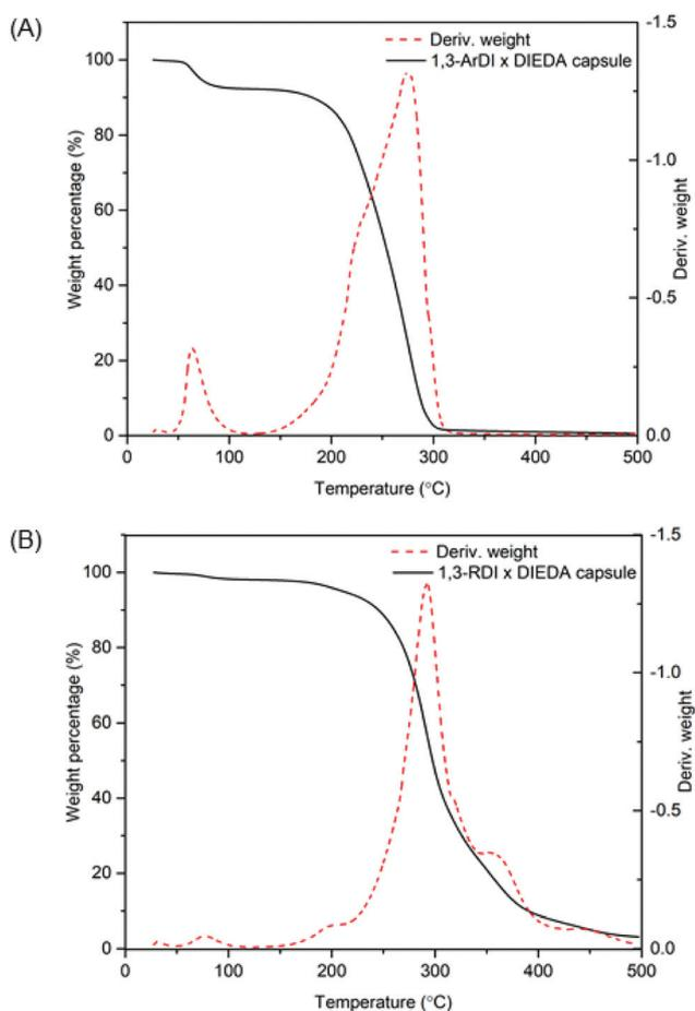
Fig. 5 TGA weight loss profiles and their first derivatives of (A) 1,3-ArDI-DIEDA capsules and (B) 1,3-RDI-DIEDA capsules.
